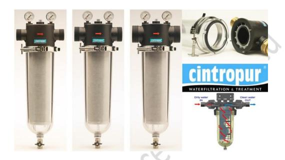
The Cintropur design is innovative in two ways. The flow of water entering the system is transformed into a vortex using a centrifugal vane, which forces large particles to the base of the bowl to enable purging of solids via the drain cock. The exclusive Cintropur filtration sleeve performs secondary filtration depending on the micron size selected (ranging from  $25\mu$  to  $100\mu$ ).
